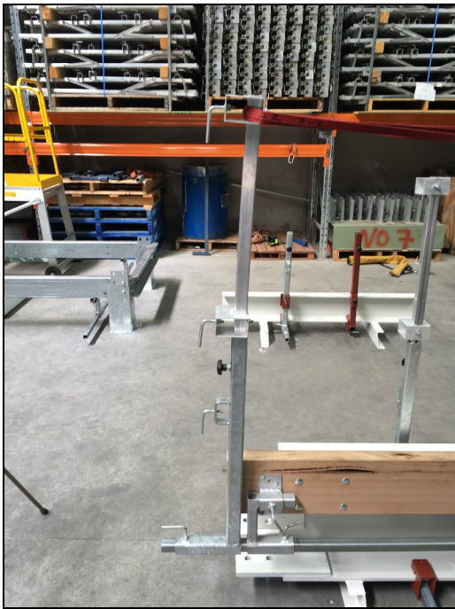
Figure 15: Timber beam clamp with offset bracket (C design), 660mm steel base and aluminium post
