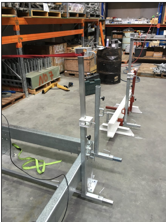
Figure 1: Offset bracket (Z design) with C-purlin clamp, 660mm steel base and aluminium post
