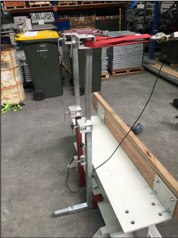
Figure 11: Beam clamp with 660mm steel base and aluminium post
