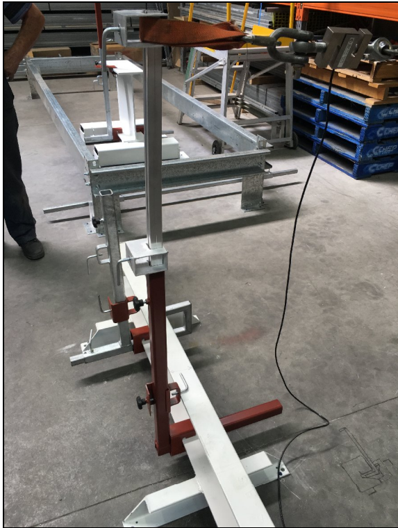
Figure 18: Beam clamp with long tail 660mm steel base and aluminium post
