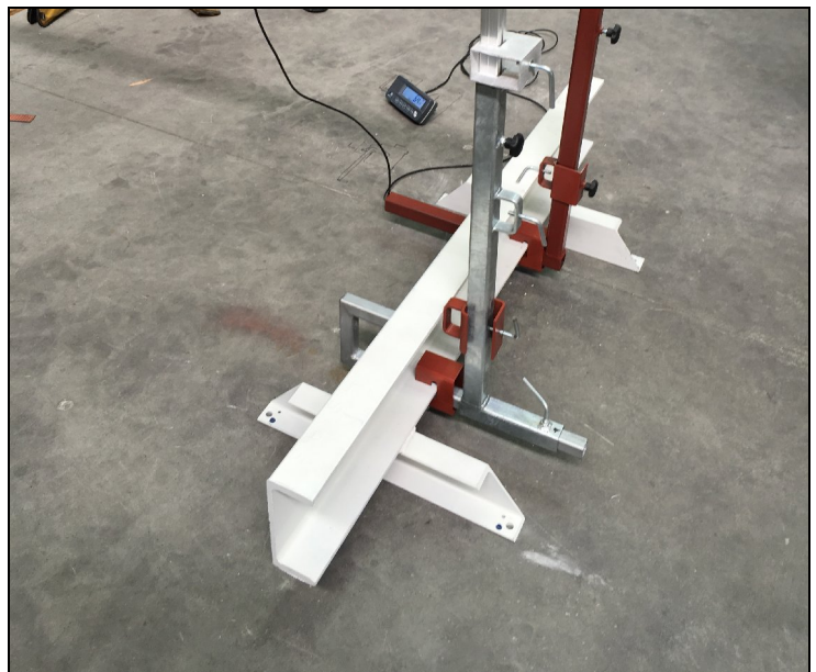
Figure 21: PFC beam test rig
