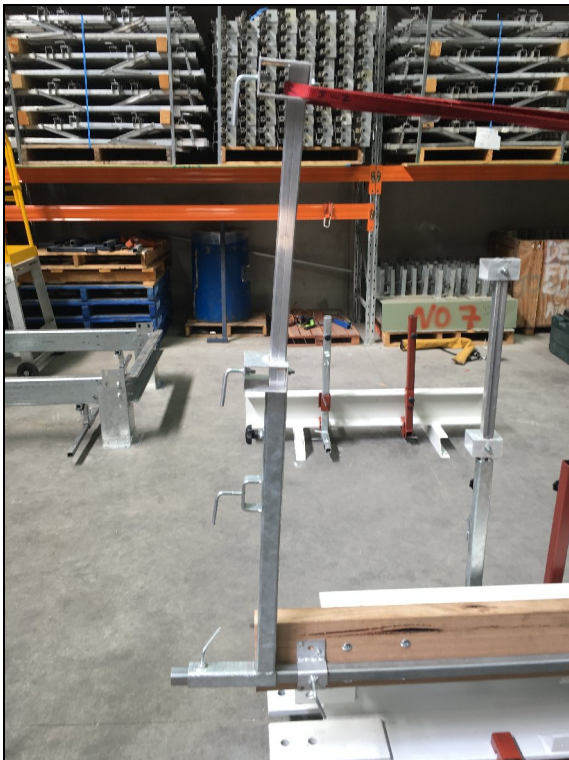
Figure 13: Timber beam clamps with 660mm steel base and aluminium post
