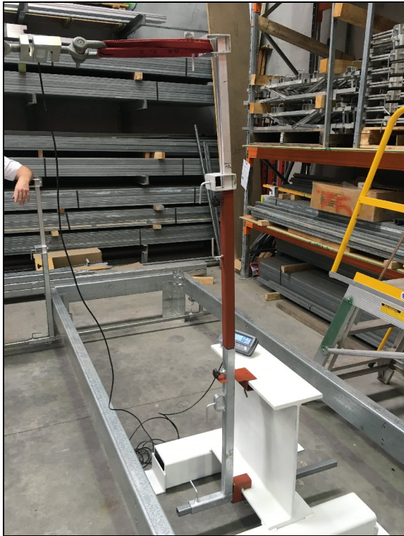
Figure 5: Beam clamp with 660mm steel base, 600mm extension bar and aluminium post
