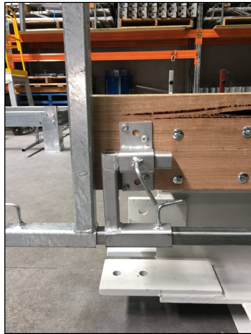
Figure 16: Timber beam clamp with offset bracket (C design)
