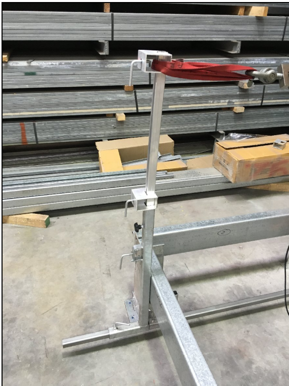
Figure 7: Offset bracket (C design) with C-purlin clamp, 660mm steel base and aluminium post
