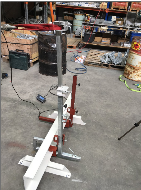
Figure 9: PFC beam clamp with 660mm steel base and aluminium post
