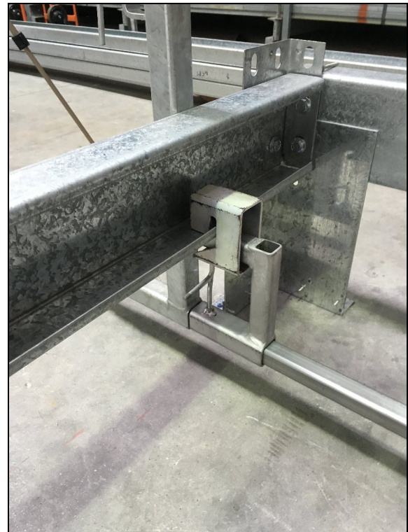
Figure 8: Offset bracket (C design) with C-purlin clamp
